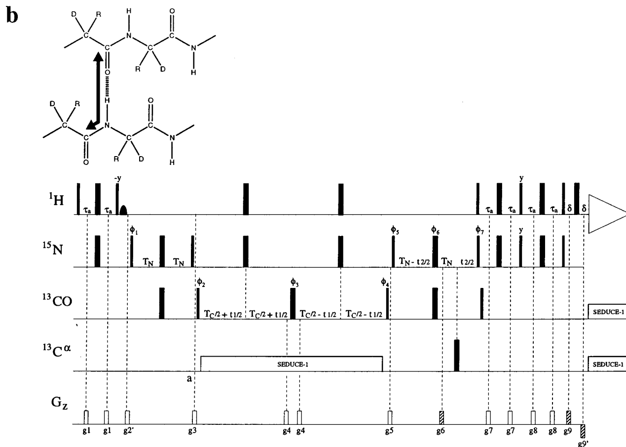
Figure 1. (Continued) — 1) dipolar and ^{13}\text{CO}(j) CSA or ^1\text{H}^{\text{N}}(i) ^{13}\text{CO}(j) dipolar and ^{13}\text{CO}(i-1) CSA interactions. The delays employed are: \tau_a = 2.3 ms, T_N = 81.7 ms, T_C = 32.5 ms (500 MHz), \delta = 250 \mu\text{s} . The phase cycle employed is: \phi_1 = (x, -x) ; \phi_2 = 2(y), 2(-y), 2(x), 2(-x) ; \phi_5 = 8(x), 8(-x) ; \phi_6 = 2(x), 2(-x) ; \phi_7 = x ; Rec = 4(x, -x), 4(-x, x) . Data sets with \phi_4 = 4(y), 4(x) and \phi_4 = \phi_4 + 90^\circ are recorded in an interleaved manner and subtracted or added to generate double- or zero-quantum data sets. The phase \phi_3 is adjusted to ensure that correlations are pure-absorptive in the F_1 frequency domain, as described for the scheme of Figure 1a. Quadrature detection in F_2 is achieved via the enhanced sensitivity approach, while quadrature is not employed in F_1 . The duration and strengths of the gradients are: g_1 = (5 ms, 5 G/cm), g_2 = (1 ms, 15 G/cm), g_3 = (1 ms, 18 G/cm), g_4 = (0.25 ms, 12 G/cm), g_5 = (0.7 ms, 20 G/cm), g_6 = (1.25 ms, 30 G/cm), g_7 = (0.4 ms, 2.9 G/cm), g_8 = (0.3 ms, 5 G/cm), g_9 = (62.5 \mu\text{s} , 27.6 G/cm). In both sequences decoupling is interrupted during application of the gradients. 75 Pulse sequences are available upon request.
